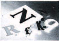
④ Sign letters cut from various plastics using a 200W CO<sub>2</sub> laser
